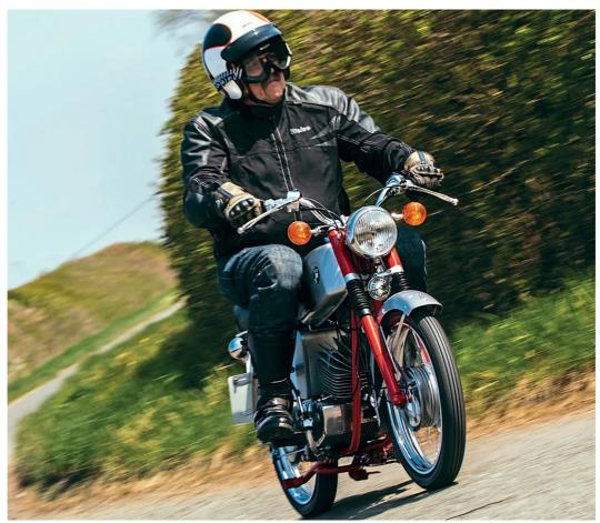
The bike has elements of both the old and new about as it moved towards the 1970s. By then even the Japanese had grasped that motorcycle theft could be an issue, yet Puch saw no reason to fit an ignition switch, instead gifting the M125 just a kill button. Perhaps, a little perversely, the bike runs plastic side-panels, yet the air-box they cover is made from cast alloy; you begin to realise that this most definitely is not your average, humble, pre-mix commuter.
